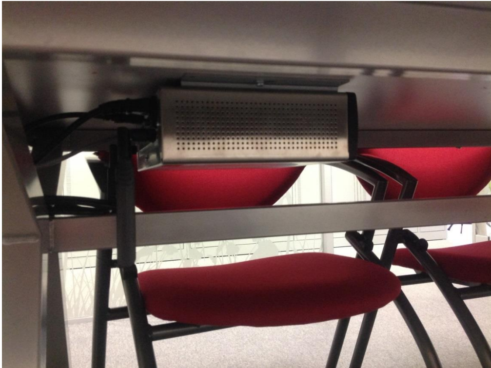
Figure 7: Example of correct ClickShare base unit installation
