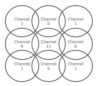
Figure 4: Theoretical Wi-Fi channel allocation map
