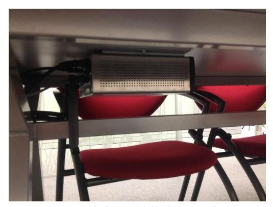
Figure 7: Example of correct ClickShare base unit installation
